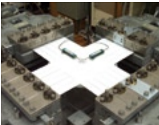
Biaxial Tensile Test We measure the tensile stiffness and the Poisson ratio from the result of the relation of the stress-strain when the material is slowly pulled in a biaxial direction.
