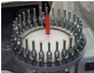
Creep test by hydraulic control method We measure the creep rupture of the materials by water pressure, keeping membrane surface with uniform tension in all directions.
