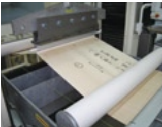
Tensile Test for Clamping It is necessary to measure the clamping strength of membrane panels for the design of membrane structures. We evaluate clamping strength by using the large-load type tensile tester.
