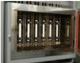
Creep Test We measure strain and the presence or absence of breaking in the material by applying a constant tensile load over a long period of time at a constant temperature.
