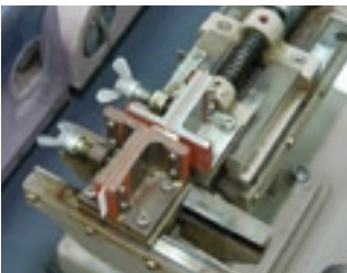
Resistance to Folding and Abrading Test We evaluate the change in appearance and ease of peeling of the coating due to folding and abrading.
